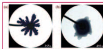
*Fig.1: Displacement of a solution of polymer by dyed water: (a) in absence of any reaction, viscous fingering is observed because of the unfavorable viscosity gradient; (b) in presence of a chemical reaction decreasing the viscosity in the reactive zone at the miscible interface between water and the polymer, a reduction of the fingering instability and hence a more efficient displacement is obtained.*
